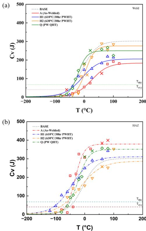
Fig. 2. Charpy ductile-brittle transition curves : (a) Weld, (b) HAZ
