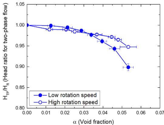
Fig. 2. Head degradation according to the void fraction
