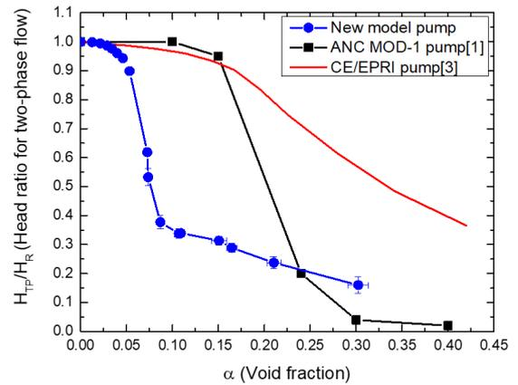
Fig. 3. Comparison of the head degradation under two-phase flow conditions for several reactor coolant pumps
