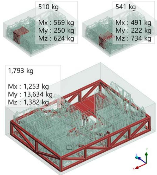
Fig. 5 Structural mass and hydraulic mass
