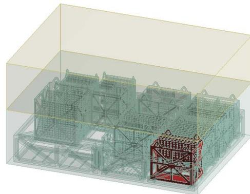
Fig. 2 Acoustic region and acceleration exciting surface for a rack (rack01)
