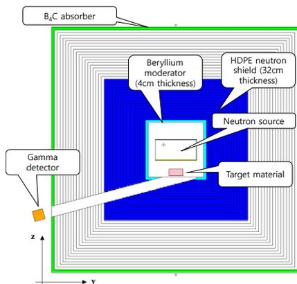
Fig. 8 Gamma Detection Passage Oriented at  $-15^\circ$  to the Y-Axis (Case B)
