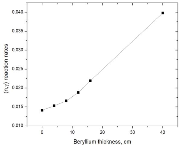
Fig. 6 Variation in (n,γ) reaction rate as a function of beryllium thickness
