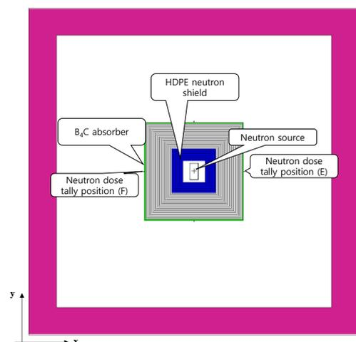
Fig. 2 Description of the MCNP Model at x-y plane
