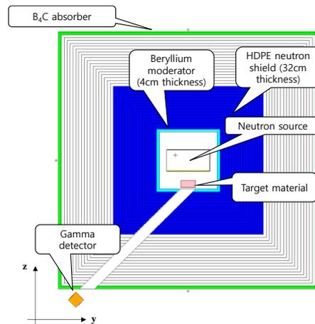
Fig. 9 Gamma Detection Passage Oriented at  $-45^\circ$  to the Y-Axis (Case C)
