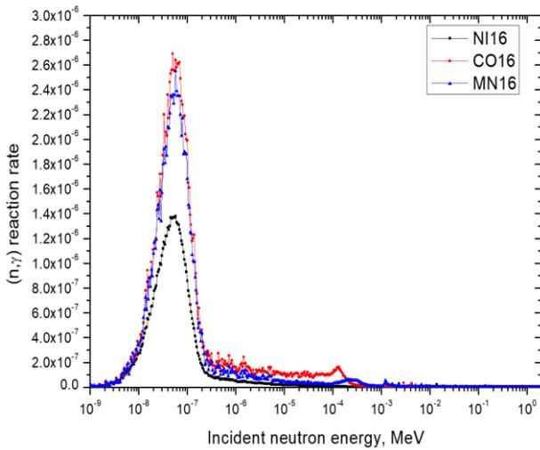
Fig. 4 neutron capture reactions for various target materials
