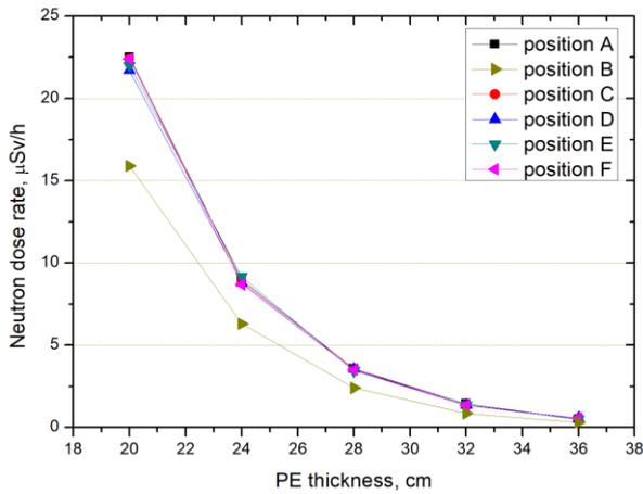
Fig. 3 Neutron dose rate according to the HDPE thickness
