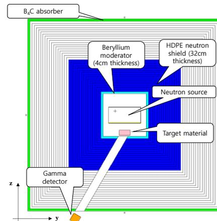
Fig. 10 Gamma Detection Passage Oriented at  $-60^\circ$  to the Y-Axis (Case D)
