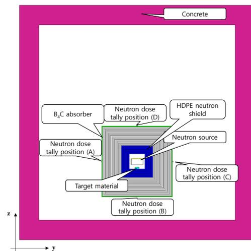
Fig. 1 Description of the MCNP Model at y-z plane
