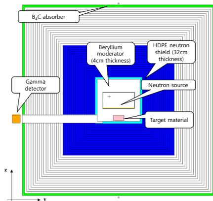
Fig. 7 Gamma Detection Passage Aligned Parallel to the Y-Axis (Case A)
