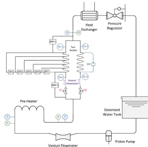
Fig. 1. Schematic diagram of experimental facility [10].
