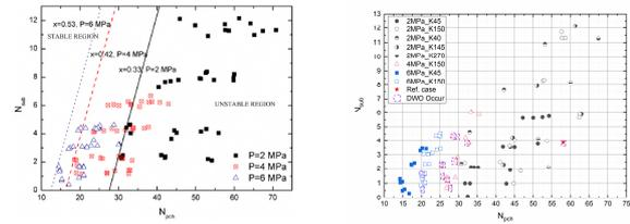
Fig. 4. Comparison stability map of calculation results with experimental data [10].
