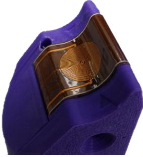
Fig. 2. Flexible PCB coil mounted on concave probe housing
