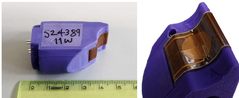
Flexible PCB coil mounted on concave probe housing
