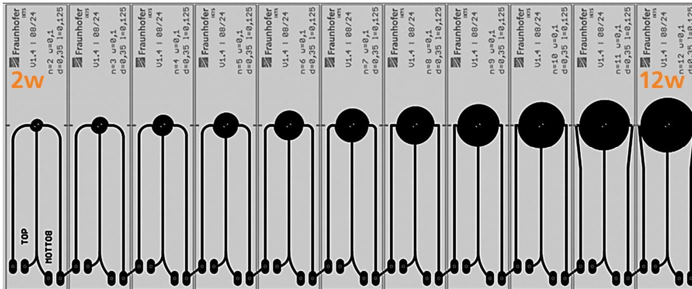
Layout of circular coils printed as flexible PCBs.
