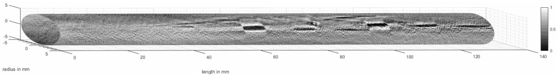
Eddy-current scan of cracks in chrome layer
