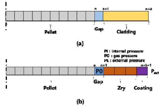
Fig. 1. Mechanical analysis model [6]: (a) existing model, (b) enhanced model for ATF.
