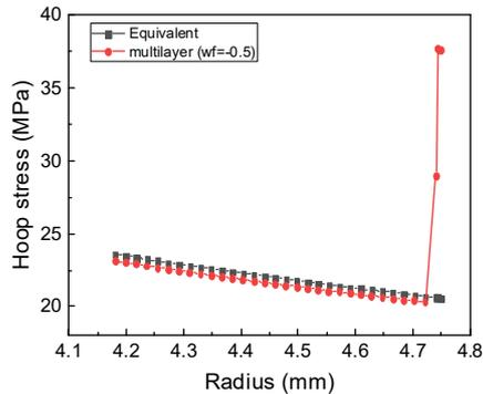
Fig. 5. 'Multilayer' calculation results with the equivalent and multilayer model (hoop Stress comparison).
