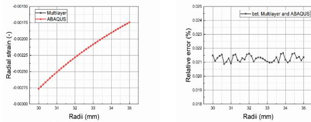
(a) Radial strain comparison (Elastoplastic) (b) Relative displ. error (Elastoplastic)
