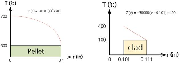
a) Temperature gradient of the pellet (b) Temperature gradient of the cladding
