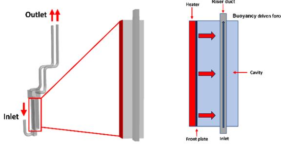
Fig. 2. Heat Transfer and Air Flow Path in the NSTF
