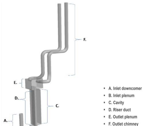
Fig. 1. Schematic of overall NSTF
