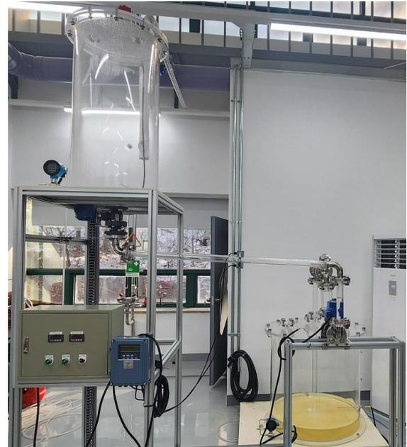
Fig. 1. K-MSR drain system scaled experimental apparatus
