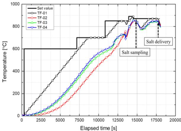
Fig. 3. Salt and crucible temperatures during the melting and delivery process
