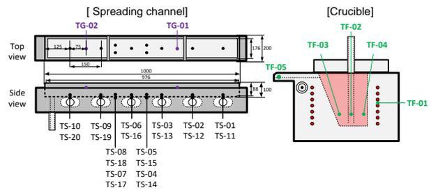
Fig. 2. Thermocouple install locations
