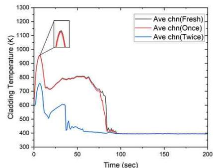
Fig. 5. Cladding temperature of average core rods with the same fresh fuel gap gas composition
