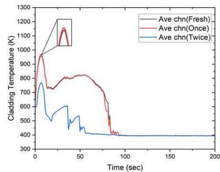
Fig. 3. Cladding temperature of average core rods by burnup
