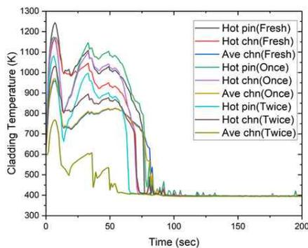
Fig. 2. Cladding temperature calculation results for OPR1000 during the LBLOCA
