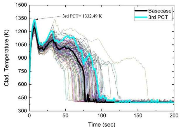
Fig. 7. Results of 124 uncertainty calculations of cladding temperature in hot pin (fresh fuel)
