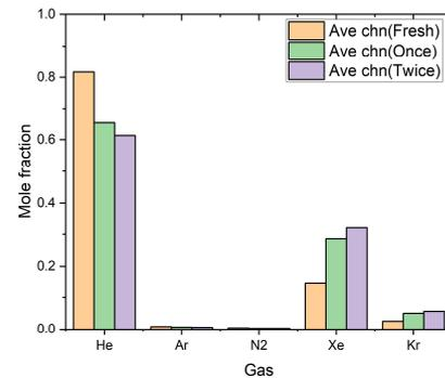
Fig. 4. Gap gas composition of average core rods by burnup
