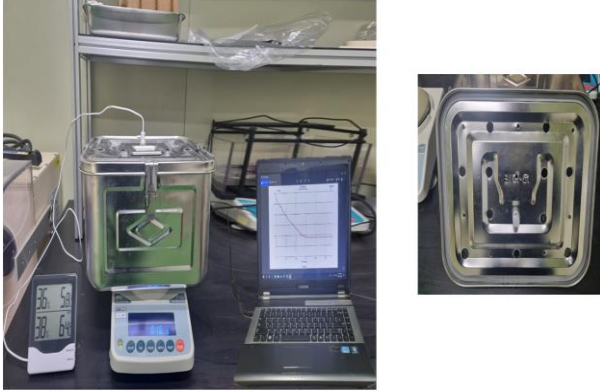
Fig 1. Real-time evaporation measurement system (left) Lid and holes of the wet drying container (right)
