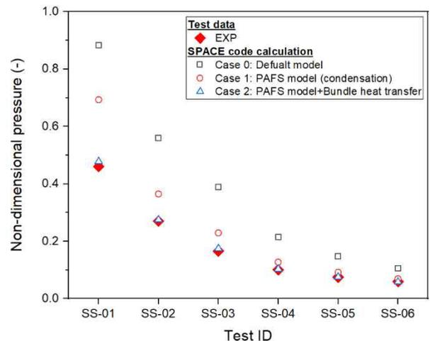
Fig. 3. Steam pressure of SPACE code calculation for LAPLACE experiments
