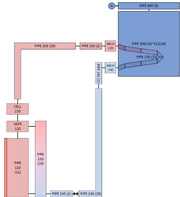
Fig. 2. Nodalization of SPACE code input model for LAPLACE test facility
