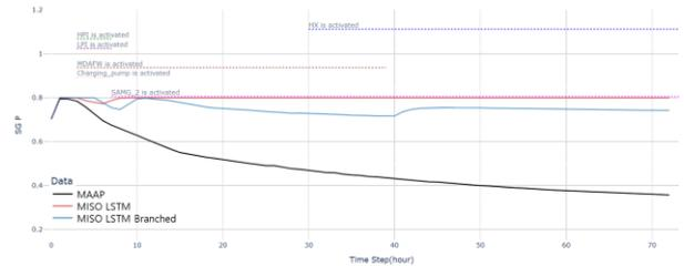
**Figure 7. Steam Generator Pressure Trends in Scenarios with Poor Predictive Performance**
