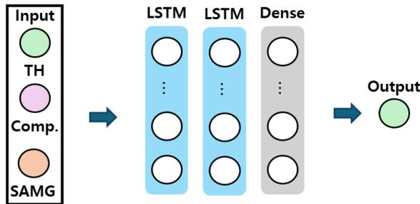
Figure 3. Diagram of Non-branched Model
