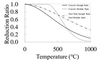
Fig. 3. Strength reduction ratio by temperature
