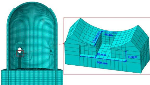
Fig. 2. Geometrical properties for postulated void
