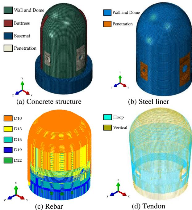
Fig. 1. FE model of 1:4 scale PCCV
