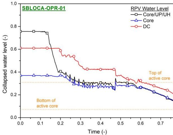
Fig. 3. Collapsed water level in the RPV
