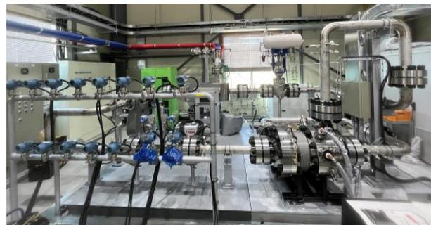
Fig. 1. Experimental facility for sCO<sub>2</sub> two-stage high-pressure ratio centrifugal compressor
