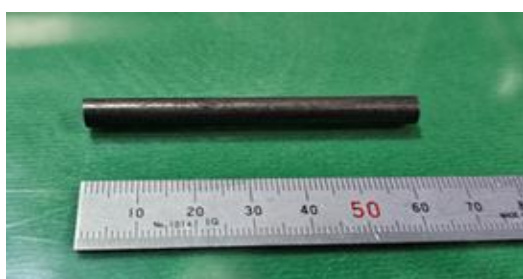
Fig. 2. Fabricated annular fuel using injection casting
