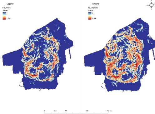
Fig. 2. Factor of safety index map when  $m = 0$  and  $m = 1$ .
