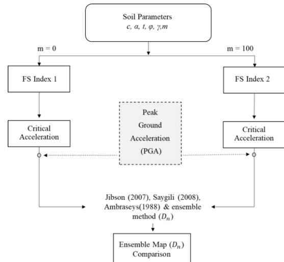
Fig. 1. Workflow illustrating the process for creating a landslide susceptibility comparison map.
