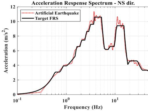
Fig. 4. Input acceleration response spectrum (NS dir.)
