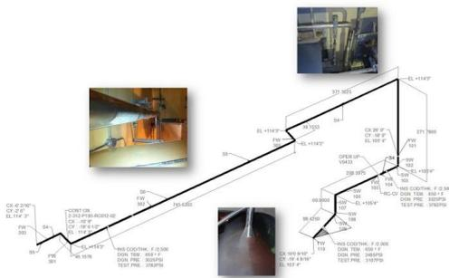
Fig. 1. ISO drawing and main part shapes of target piping [2]
