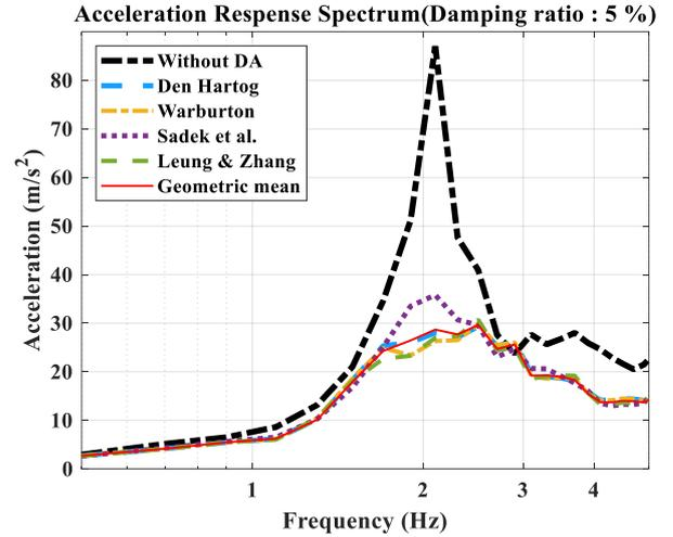
Fig. 5. Acceleration response spectrum comparison at the DA installation location (damping ratio: 5%)
