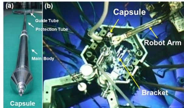
Fig. 1. HANARO irradiation capsule: (a) Irradiation capsule and (b) a capsule system installed in the reactor core.
