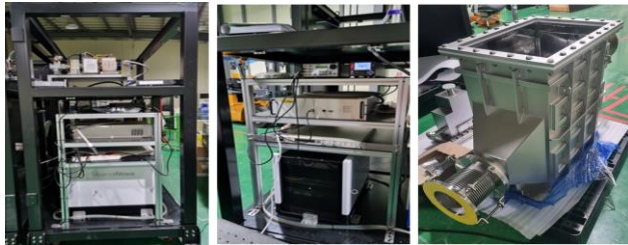
Figure 3. Developed electron accelerator power(left), control unit(middle), electron beam gas reactor(right)
