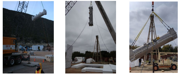
(a) 9m-10° drop (b) 9m-90° drop (c) 1m-Puncture Fig.5 Configuration of PIONEER G HAC drop tests
