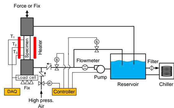
Fig. 1. Schematic Diagram of tests system
