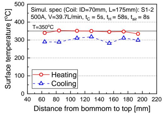
Fig. 3. Thermal fatigue during heating and cooling temperature distribution at the specimen surface
