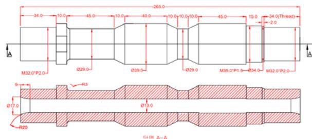
Fig. 2. Simulated specimen shape for thermal fatigue testing
