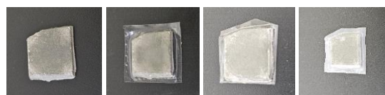
Fig. 1. NTD-Ge samples w/o and w/ packaging materials (sealing film, transparent tape, and opaque tape, from left).
