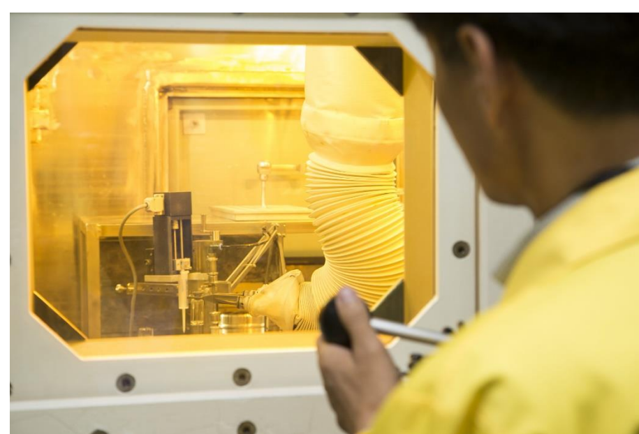
Hot cell at KAERI
