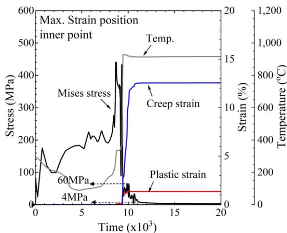
Fig. 1. Time-dependent changes in equivalent stress, inelastic strain, and temperature at the inner wall surface point at the maximum strain position.
