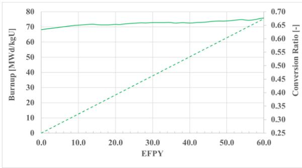
Figure 6. Burnup and conversion Ratio for KCl-UCl<sub>3</sub>-UF<sub>4</sub> (15% enrichment) w/ BA
