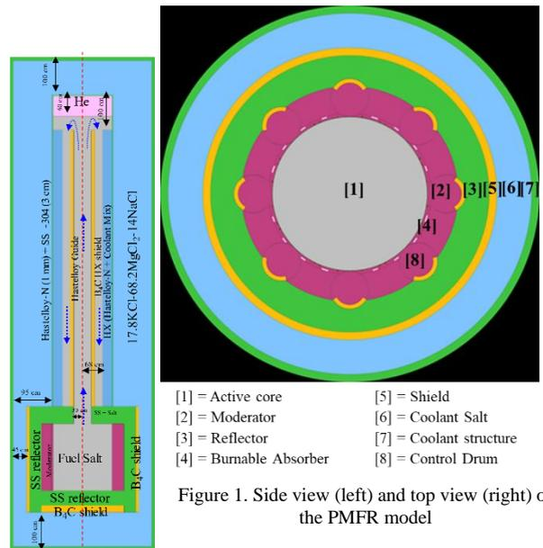
Figure 1. Side view (left) and top view (right) of the PMFR model
