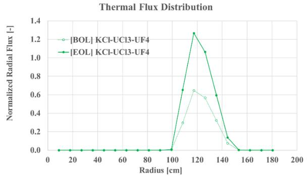
Figure 9. Radial thermal flux distribution
