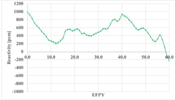
Figure 5. Detailed depletion result for KCl-UCl<sub>3</sub>-UF<sub>4</sub> (15% enrichment) w/ BA
