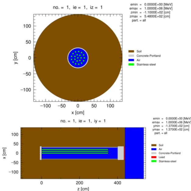
Fig. 4 Geometry in XY and XZ axis
