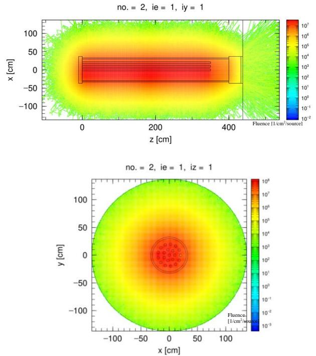
Fig. 5 Particles fluence distribution for photons
