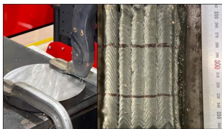
Fig. 2. OFC 3-layer deposition using a Tandem system
