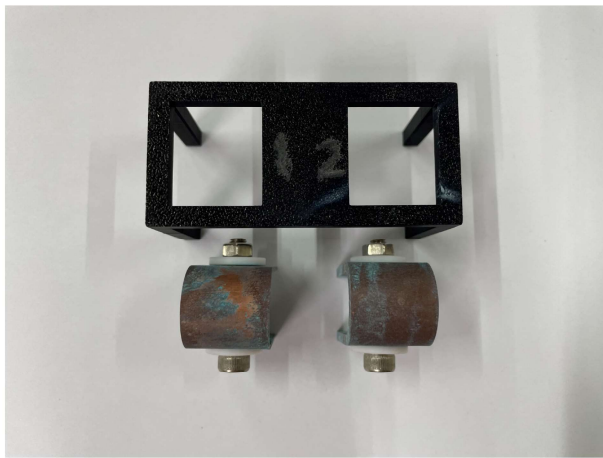
Figure 1 . U-bend Cu specimens after 6 months immersed in KURT underground water. Left: 1 mm thickness; Right: 2.5 mm thickness.
