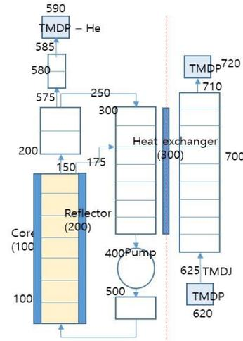
Fig. 1. The MARS nodalization for a conceptual MSR design
