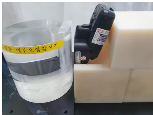
Figure 1. Measurement geometry (RadEye B20-ER)
