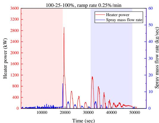
Fig. 9. PPCS operation vs. time under 100-25-100% load-following operation with ramp rate of 0.25%/min.
