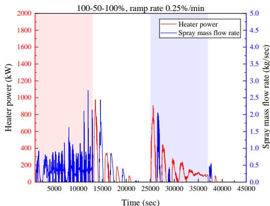
Fig. 5. PPCS operation vs. time under 100-50-100% load-following operation with ramp rate of 0.25%/min. The red-shaded region denotes the ramp-down zone, while the blue-
