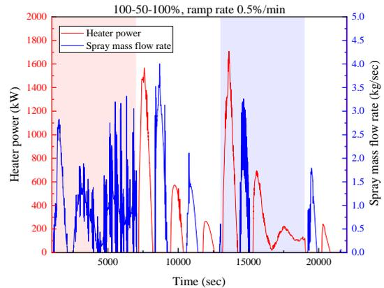
Fig. 6. PPCS operation vs. time under 100-50-100% load-following operation with ramp rate of 0.5%/min.
