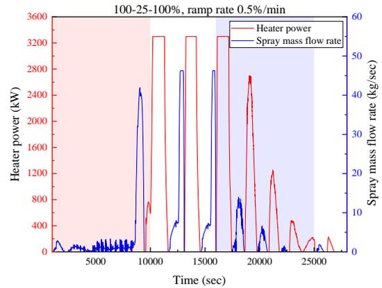
Fig. 10. PPCS operation vs. time under 100-25-100% load-following operation with ramp rate of 0.5%/min.
