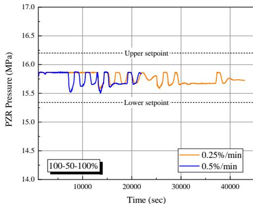
Fig. 4. Pressurizer pressure vs. time under 100-50-100% load-following operation with different ramp rates.
