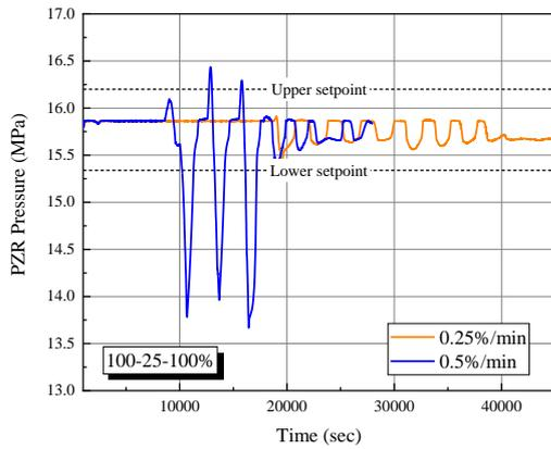
Fig. 8. Pressurizer pressure vs. time under 100-25-100% load-following operation with different ramp rates.
