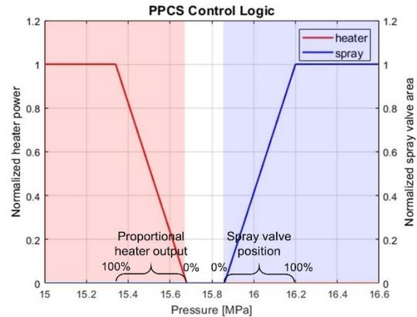
Fig. 2. PPCS control logic. The red-shaded region denotes the heater's operating zone, while the blue-shaded region denotes the spray's operating zone.
