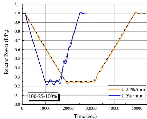
Fig. 7. Reactor power vs. time under 100-25-100% load-following operation with different ramp rates. The black dashed lines denote the target reactor power value.
