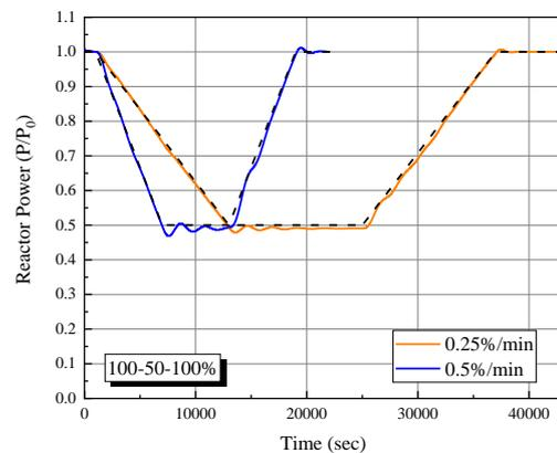
Fig. 3. Reactor power vs. time under 100-50-100% load-following operation with different ramp rates. The black dashed lines denote the target reactor power value.
