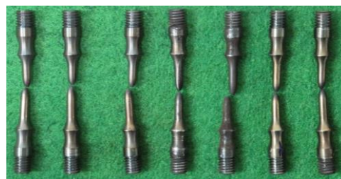
Figure 4. Specimens after the creep tests
