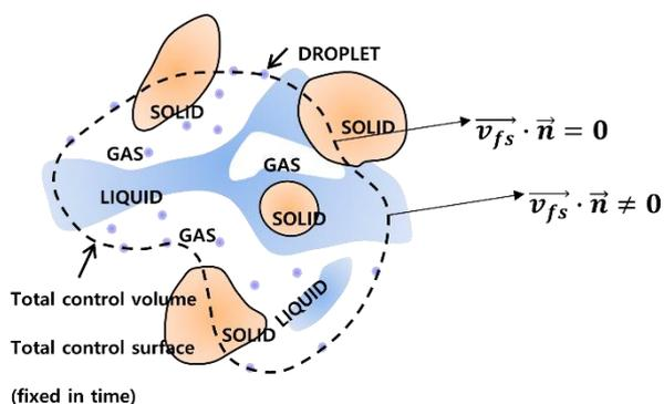
Fig. 2. Porous media control volume scheme
