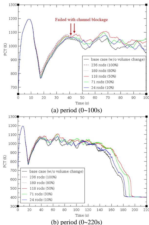
Fig. 3. Sensitivity results – effect of channel deformation on PCT behavior of hot pin
