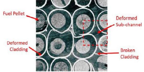
Fig. 1. Rod bundle cross-section after PHEBUS LOCA experiment [1]
