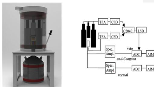
Fig. 1. Compton Suppression system (a) and block diagram of the signal processing system (b)
