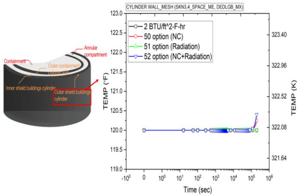
Figure 9. Outer shield buildings cylinder surface temperature
