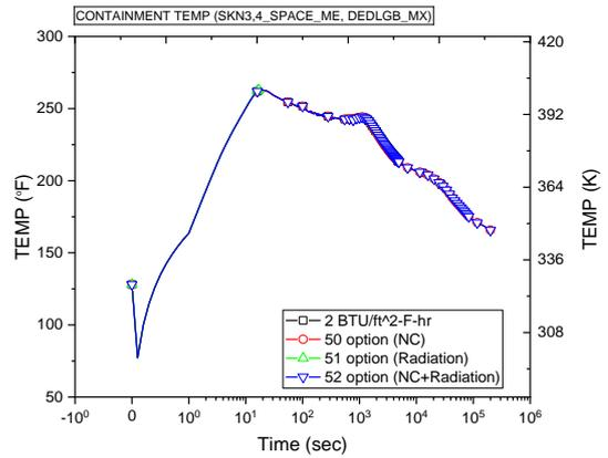
Figure 11. Containment temperature when the containment wall was changed from concrete to carbon steel
