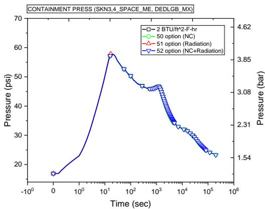
Figure 10. Containment pressure when the containment wall was changed from concrete to carbon steel
