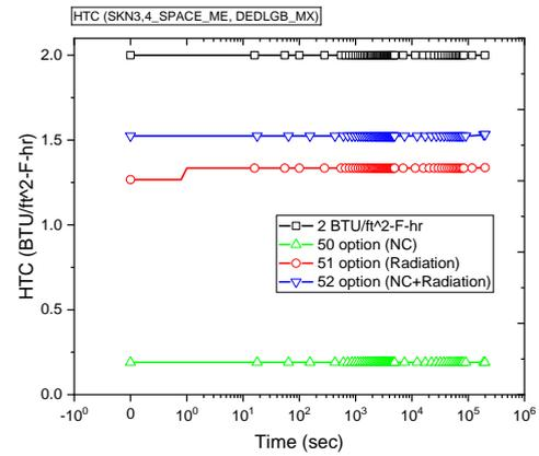
Figure 7. Outer containment cylinder wall HTC using CONTEMP-LT/028
