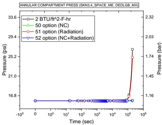
Figure 5. The annular compartment pressure by HTC model using CONTEMP-LT/028
