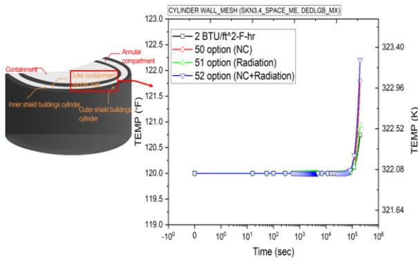
Figure 8. Outer containment cylinder wall surface temperature
