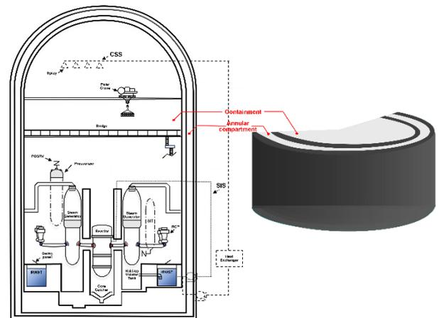
**Figure 1. Schematic of Korea NPPs' APR1000 double containment.**
