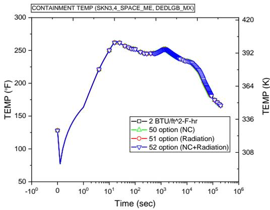
Figure 4. Temperature of containment by HTC model using CONTEMP-LT/028
