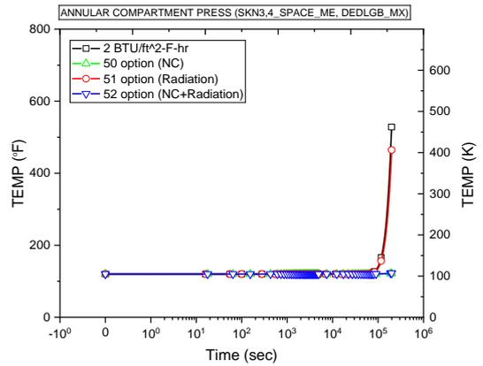
Figure 6. The annular compartment temperature by HTC model using CONTEMP-LT/028
