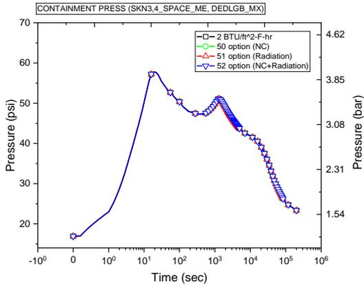
Figure 3. Pressure of containment by HTC model using CONTEMP-LT/028
