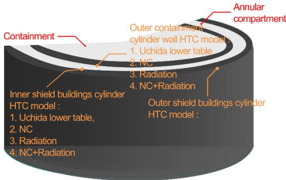
**Figure 2. Scope of HTC model double containment using CONTEMPT-LT/028**
