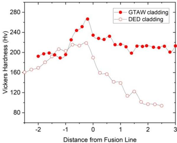
Fig. 2. Comparison of Vickers hardness profiles near clad layer formed by GTA welding and clad layer formed by laser deposition.
