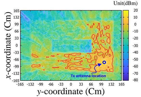
(a) Path gain distribution derived from an EM simulator.
