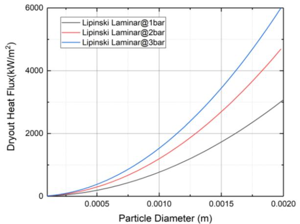
Fig. 4. Lipinski Laminar 0-D(1982) Dry-out Heat Flux at 1,2,3 bar and  $\epsilon = 0.47$
