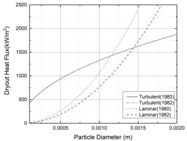
Fig. 3. Lipinski's 0-D Model 1980 vs 1982 at 1bar and  $\epsilon = 0.47$
