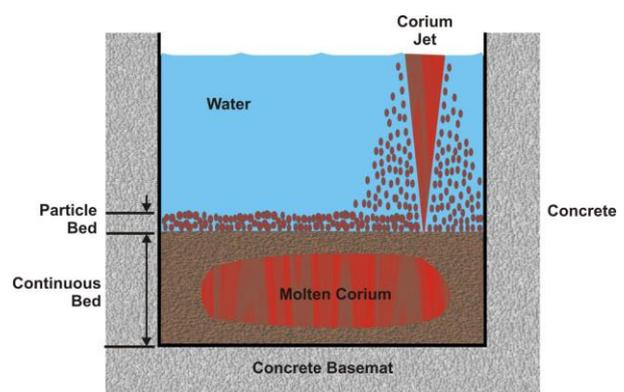
Fig. 1. Illustration of particle bed generation through jet breakup [1]
