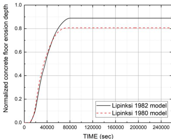
Fig. 5. Normalized concrete floor erosion depth
