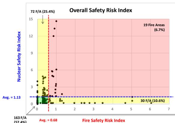
Fig. 8. Example Graph showing the Fire & Nuclear Safety Risk of OPR-1000 NPP on simultaneously 2 axes
