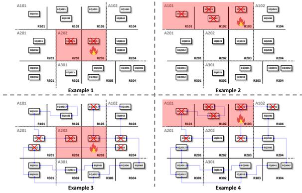
Fig. 3. Example of affected equipment in the event of a fire for fire area
