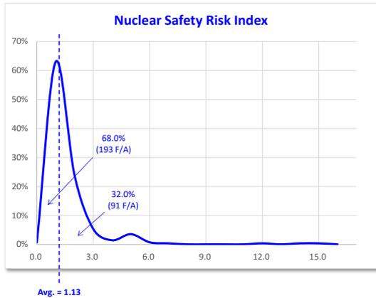
Fig. 7. Example of a Nuclear Safety Risk Distribution of OPR-1000 NPP
