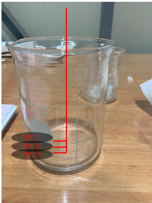
Fig. 3. Beaker for water containment and placement of Thermocouples (TC) with intervals.
