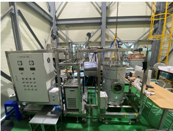
Fig. 1. Lab-scale vacuum drying test setup overview.
