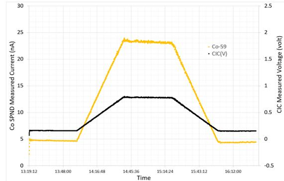
Fig. 5. Constant rate power ascending & descending
