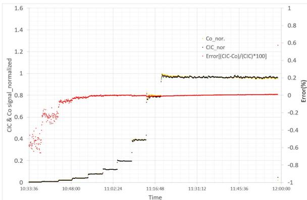
Fig. 4. CIC vs. Co-59 SPND signal normalized error
