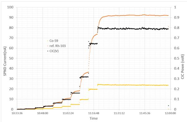
Fig. 3. SPND signal trend during power ascending
