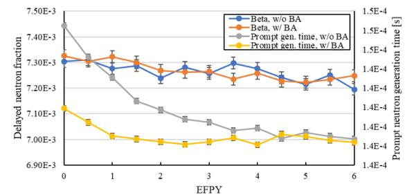
Fig. 7. Effective delayed neutron fraction and adjoint-weighted prompt neutron generation time vs full-power operation time with and without BA.
