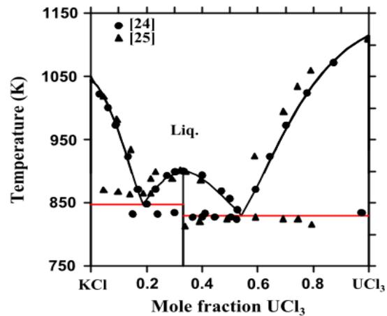
Fig. 1. Phase diagram of KCl-UCl<sub>3</sub> [3]
