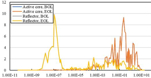
Fig. 8. Neutron spectrum in the active core and reflector in BOL and EOL.
