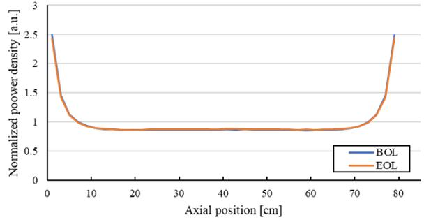
Fig. 9. Axial power distribution.
