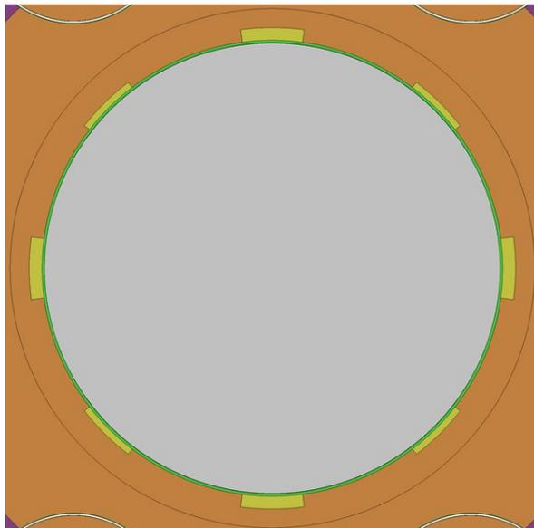
Fig. 4. Location and shape of burnable absorber (not in scale)
