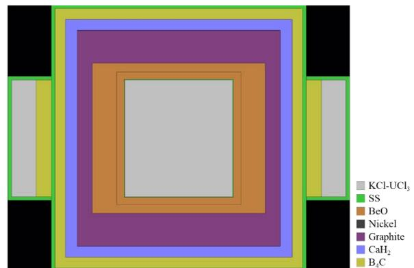
Fig. 2. Side view of micro MSR
