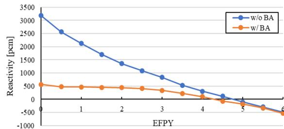
Fig. 5. Reactivity vs full-power operation time with and without BA.
