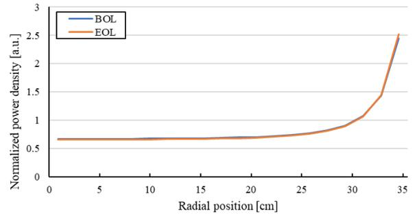
Fig. 10. Radial power distribution.
