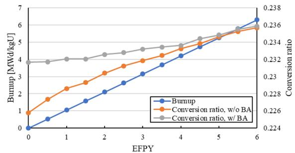
Fig. 6. Burnup and conversion ratio vs full-power operation time with and without BA.
