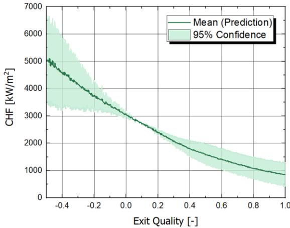
Fig. 5. Variations of mean and 95% confidence intervals of the CHF prediction by the BNN with respect to exit quality (constant  $d_i=0.004$  m,  $p=100$  kPa, and  $G=100$  kg/m<sup>2</sup>-s)
