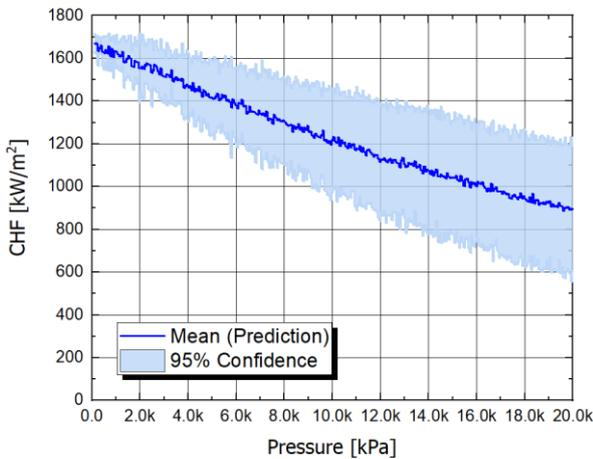
Fig. 6. Variations of mean and 95% confidence intervals of the CHF prediction by the BNN with respect to system pressure (constant  $d_i=0.004$  m,  $G=100$  kg/m<sup>2</sup>-s and  $x_{exit}=0.8$ )
