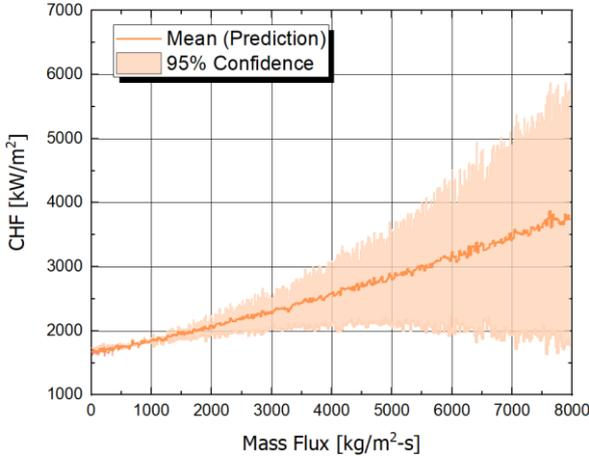
Fig. 4. Variations of mean and 95% confidence intervals of the CHF prediction by the BNN with respect to mass flux (constant  $d_i=0.004$  m,  $p=100$  kPa, and  $x_{exit}=0.8$ )
