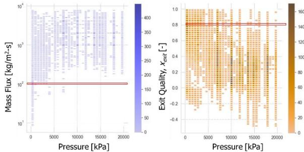
Fig. 8. 2D histograms; pressure versus mass flux and exit quality
