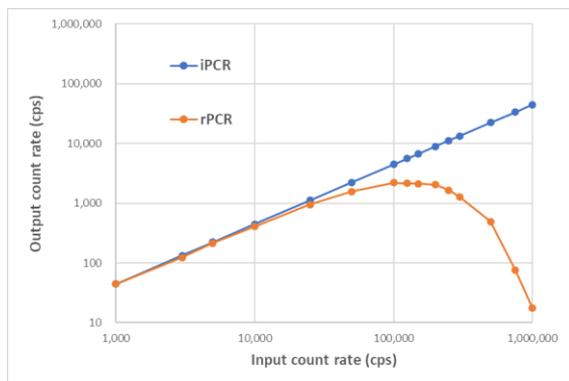
Figure 2. Peak count rates (1.33 MeV peak) according to emulated input count rate
