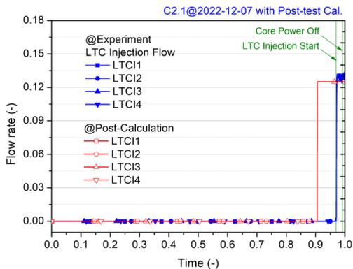
Fig. 7. Comparison of actuation timing and flow rate of LTCI
