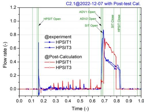
Fig. 5. Comparison of injection flow rate from HPSITs
