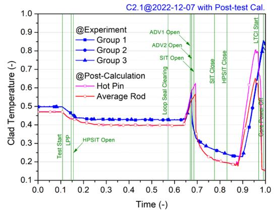
Fig. 8. Comparison of clad temperature trends
