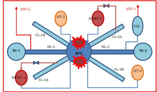
Fig. 1. Schematics of test configuration for the C2.1
