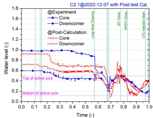
Fig. 3. Comparison of water levels in RPV
