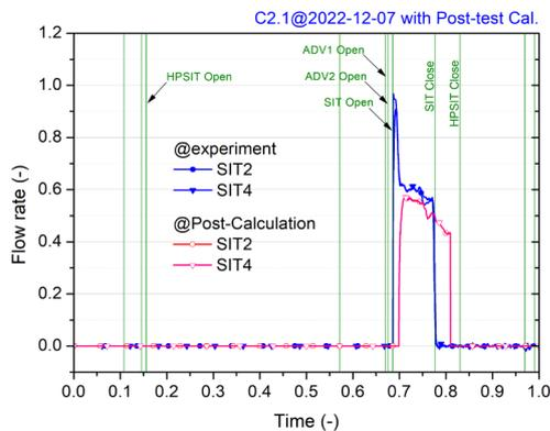
Fig. 6. Comparison of injection flow rate from SITs
