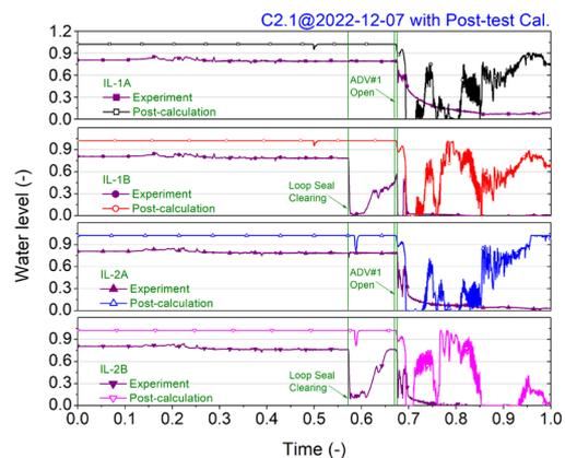
Fig. 4. Comparison of loop seal behavior in the intermediate legs
