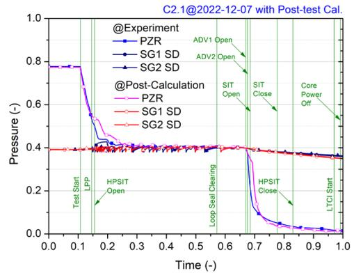
Fig. 2. Comparison of system pressure trends
