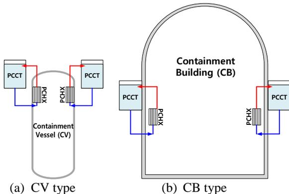
Figure 2. Conceptual diagram of PCCS installation
