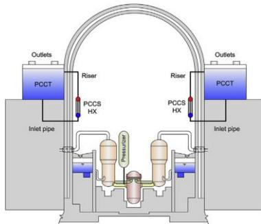
Figure 1. Schematic diagram for iPOWER PCCS [1]
